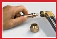
Step 1. Remove standard tip nut and worn out oxy tip.
