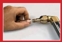
Step 3. Place selected oxy tip into tip nut and screw adaptor and tip nut with tip onto the torch.
